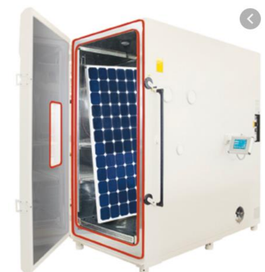
Damp heat at higher temperature 95°C instead of 85°C
